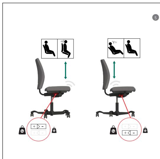
**ENG** If you cannot find your ideal setting purely by turning the wheel, you can override the default tilt tension and back height settings as shown (tilt fully forwards and backwards to engage the new settings).
